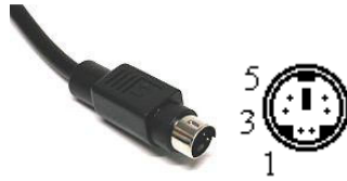
Figure 6 –PS/2 connector (Wire Side Shown)
