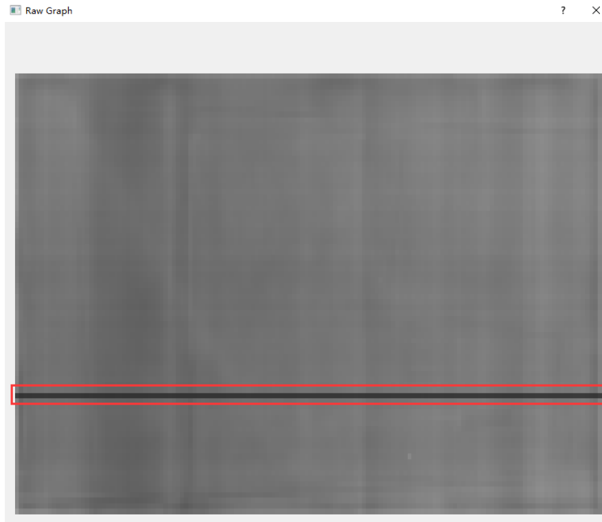
Figure 17. touch foil shot circuit
