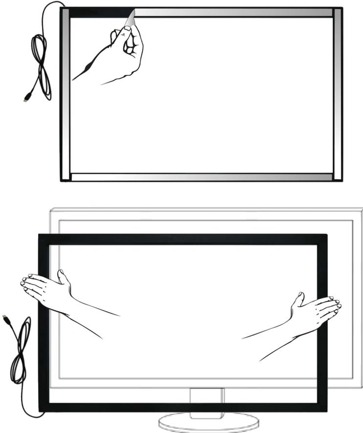
(4) After fixing the touch screen with 3M tape, please place the display on a flat plane (note: the touch screen shall be place at the bottom layer) for 24 hours.
