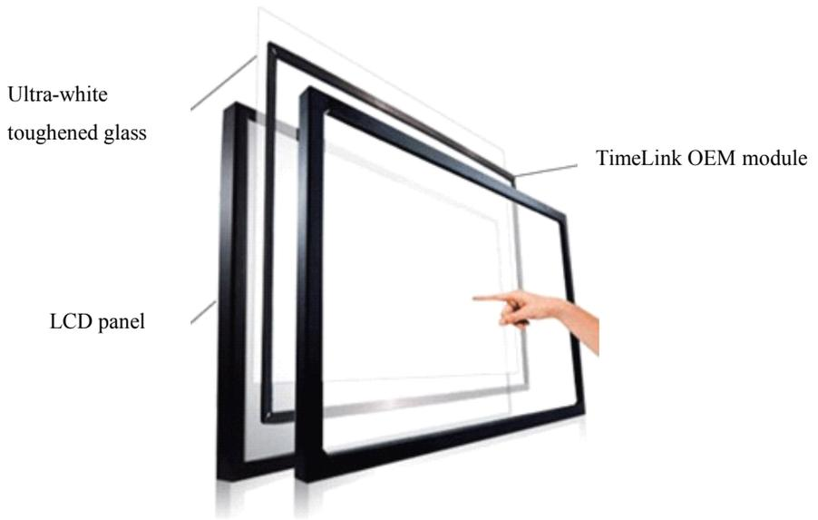
Schematic diagram of touch screen in embedded style
